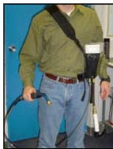
If wearing the CD2 on the chest, place the main, padded strap over your head and your arm through the loops on either side. A clip on the left side will help secure the unit and distribute the weight to the hips as well as the shoulders.
