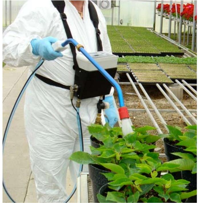
The CD2 uses a precision flow meter to accurately measure each dose. ***It is important to keep this flow meter clean by using the included filters during every use.*** Occasional cleaning of the flow meter will be necessary.
