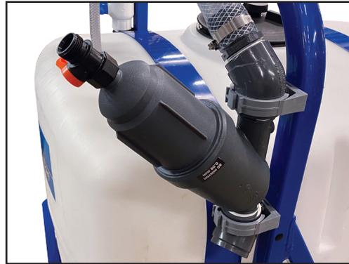
The FCST100 includes a check valve to prevent water hammer from damaging the injector. This must be used to maintain the injector warranty.
