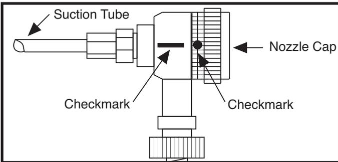
B. The nozzle cap has an O-Ring inside which may be damaged. Replace the O-Ring if it is cracked, broken or in some way damaged.
