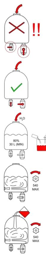
Before filling the tank, close the tank drain valve and open the pump feed line valve! The tank takes up to 400 Liters (100 gal).
