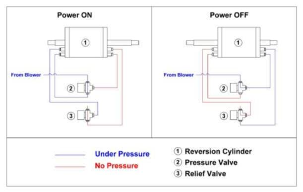
Reversion cylinder, pressure lines, valves, and their action to reverse nozzles.
