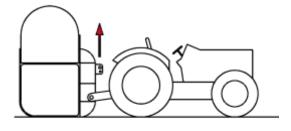
Connect the levers to the left and right hitch bolts on the TracFOG. Do not forget to secure each lever with one of the supplied cotter pins. Lift the unit slightly to facilitate the mounting of the third point rod.
