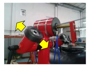
The cylinder's stroke can be set with the limiter screws shown below.
