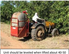
Jnit should be leveled when lifted about 40-50 cm above the ground.
