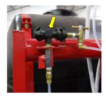
One of two anti-drip valves on the TracFOG 400 F
