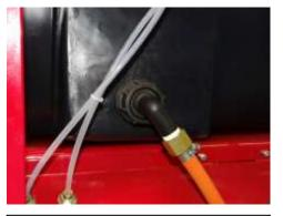
Hydraulic agitator mounted on tank
