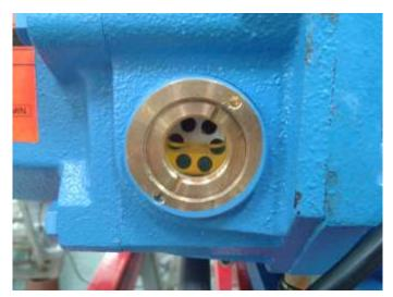
Oil level indicator showing correct oil level (filling half of the indicator).
