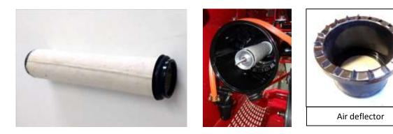
3.2.2. **FORMULATION INLINE FILTER**. The formulation inline filter is very important, as it will retain large solid particles that may find their way into the formulation tank, protecting the formulation pump. This filter should be checked and cleaned daily, which will avoid unplanned stops during application caused by obstruction of the filter. Access the filter through the right side of the machine.
