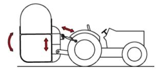
Lift and level the unit by extending or shortening the 3rd point rod. Be careful not to extend the rod too much, or it may disengage and the unit will drop. Level the unit so the PTO shaft and the input shaft of the TracFOG are on the same height and the horizontal deviation between these shafts is as little as possible.
