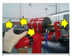
When the unit is not running, it should be possible to move the nozzles along with the piston from one side to the other by hand.
