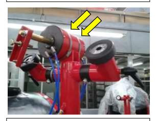
To ensure the mechanism to work properly, the cylinder must be properly fixed to the pole through the two clamps.
