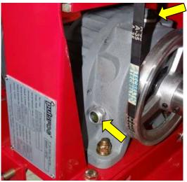
Gearbox with level indicator and refill plug.
