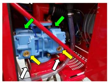
Oil level indicators (yellow arrows), oil drain tubes (white arrows) and oil fill lids (green arrows).
