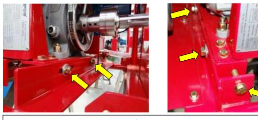
Fixing screws and screw tensioner.
