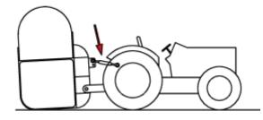
Install the 3rd point rod using the supplied 3rd point bolt. Do not forget to secure the assembly with the cotter pin.
