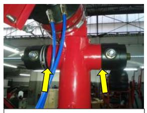
These barrels must be lubricated with **Molykote PG-75** grease. A small gap of 2 mm (arrows) between each barrel and the pole allows the barrels to rotate freely.
