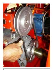
Checking the pump belt.
