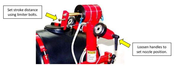
The reversion system requires compressed air from the unit's blower to operate. Run the unit to try and set the reversion stroke distance and nozzle position.
