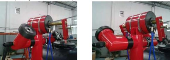
Nozzles may be pointed to left side or right side of tractor's motion.
