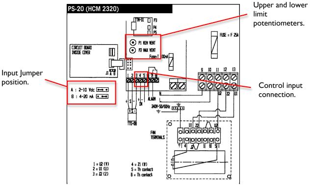
As these signals are proportional analog signals, the controller will accept the low signal as the minimum ventilation rate and the high signal as the maximum ventilation rate. As the signal increases from low to high, the controller will adjust proportionally.
