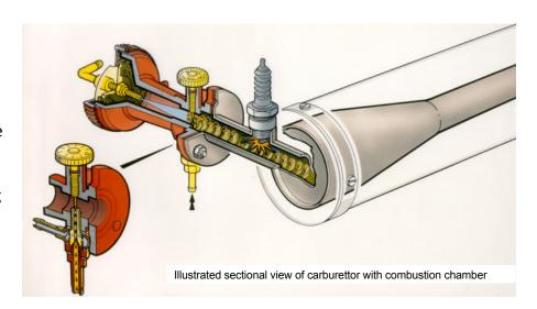
Air is pulled into the outer cooling jacket as a result of the exhaust and serves to cool the outer barrel and provide cooler air to re-condense the fog as it exits the barrel.
