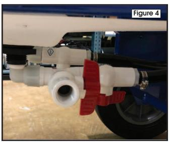
See Figure 4. Note: to drain, agitation pump must operate. This will also clean the agitation pump.
