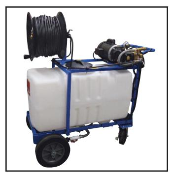
The motor has a 15.6 amp self-resetting thermal overload protection cut off. In the event of an overload, voltage drop, or over heating—the motor automatically shuts down. After a period of 3 - 4 minutes the pump can be turned on safely. The 10 foot main power cord is grounded. If you use extension cords, they should be #12 gauge grounded cords—and should not exceed 50 feet.
