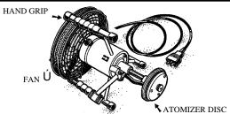
The TURBAIR ELECTRAFAN is an air-assisted spinning disc sprayer for low and ultra-low volume application of insecticides and fungicides in situations with no natural air movement, e.g. indoors. The ELECTRAFAN produces small even sized droplets which are carried in the airstream to the target.
