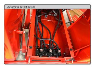
The pulsFOG K-50 is equipped with a set of safety valves, which prevent solution and/or water from flowing into the resonator if the engine stops accidentally during operation. This feature should not be used, however, for the regular shut-down. Always interrupt the fogging by closing the fog taps, not by stopping the engine!
