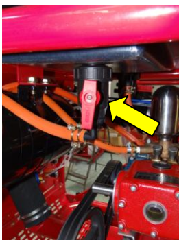
Formulation line ball valve. Must be opened for operation.
