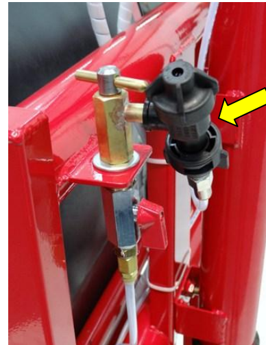
One of the anti-drip valves of the TracFOG 400
