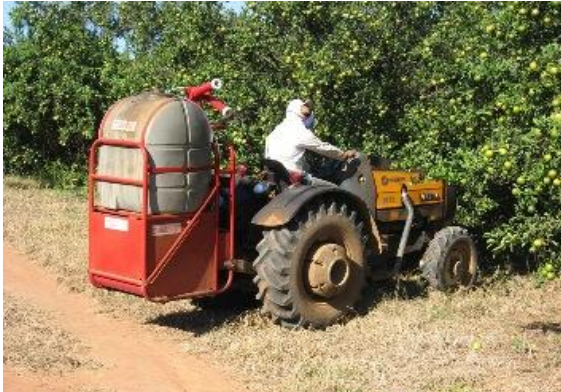
Unit should be leveled when lifted about 40-50 cm above the ground.
