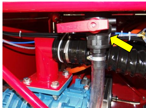
Formulation drain valve. Must be shut before filling the tank.
