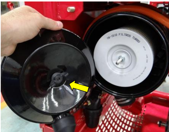
To open filter release butterfly nut.
