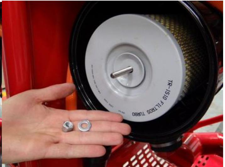
To remove element release nut.
